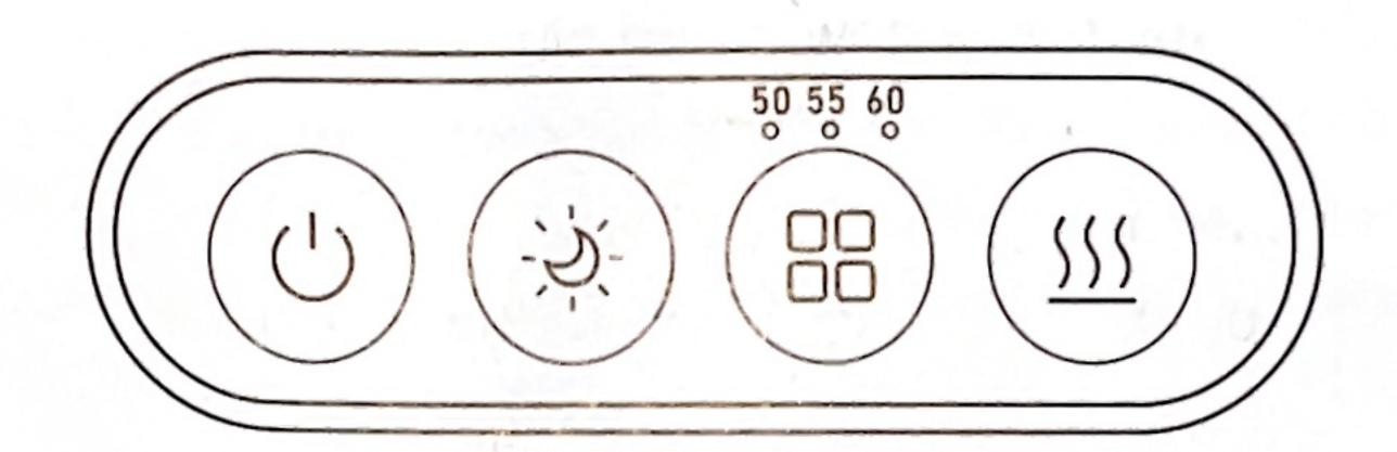
Turn on the power, the function indicator is lit and turns off after 1 second. Then turn to standby state (night light default-breathing light mode);
